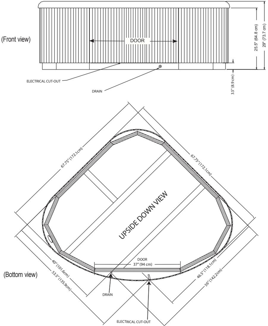
**NOTE: WATKINS WELLNESS** recommends that the TX be installed on a minimum 4" (10.2cm) thick reinforced concrete pad or structurally sound deck able to support the "dead weight" found in the spa specification chart.
