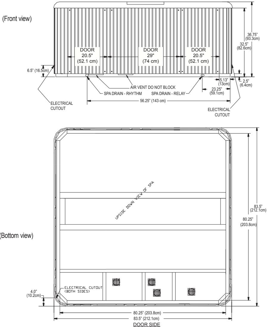
**NOTE:** WATKINS WELLNESS recommends that the Relay & Rhythm be installed on a minimum 4" (10.2cm) thick reinforced concrete pad or structurally sound deck able to support the "dead weight" found in the spa specification chart.
